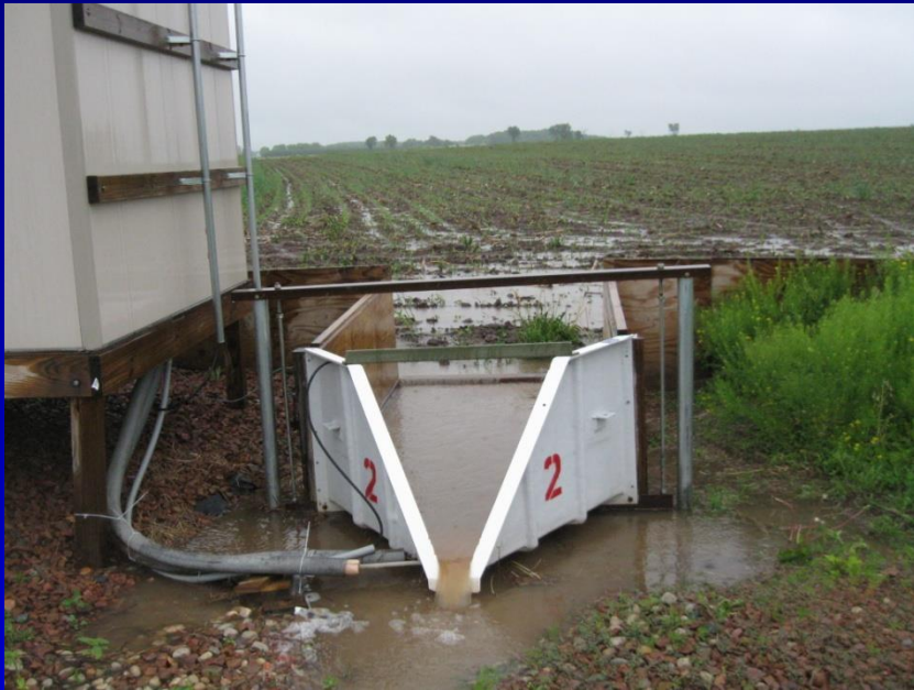
24-inch H flumes with approach channels
