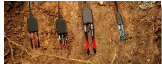
Soil moisture: How much available water? Destructive, indirect point measurement
