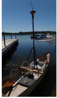
• Stream location and elevation from RTK GPS
