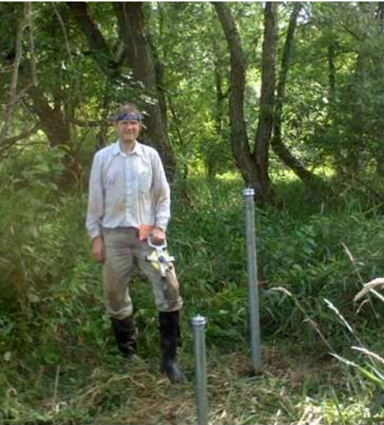
Well Points Driven at Norton Slough Floodplain
