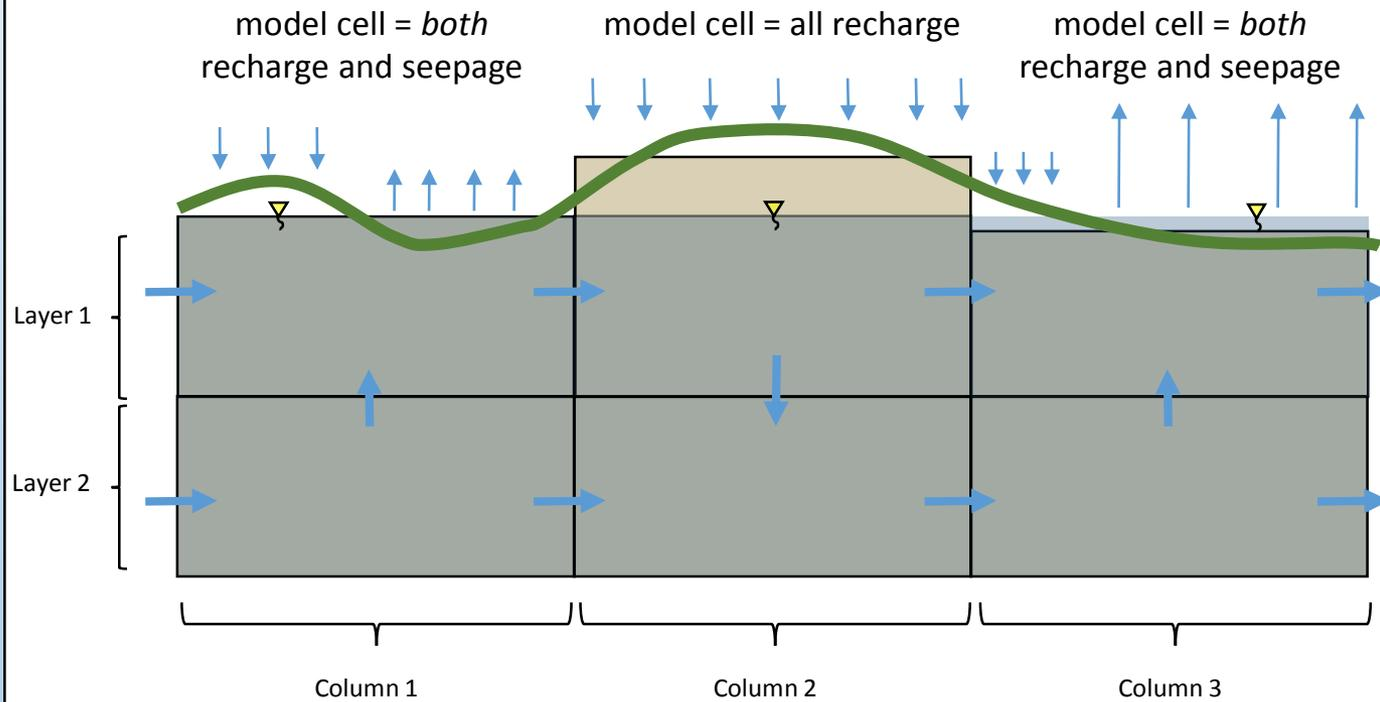
MODFLOW's UZF Package accounts for recharge *and* seepage in a single cell with the variable **SURFDEP**, which accounts for **SUR**face **DEP**ressions
