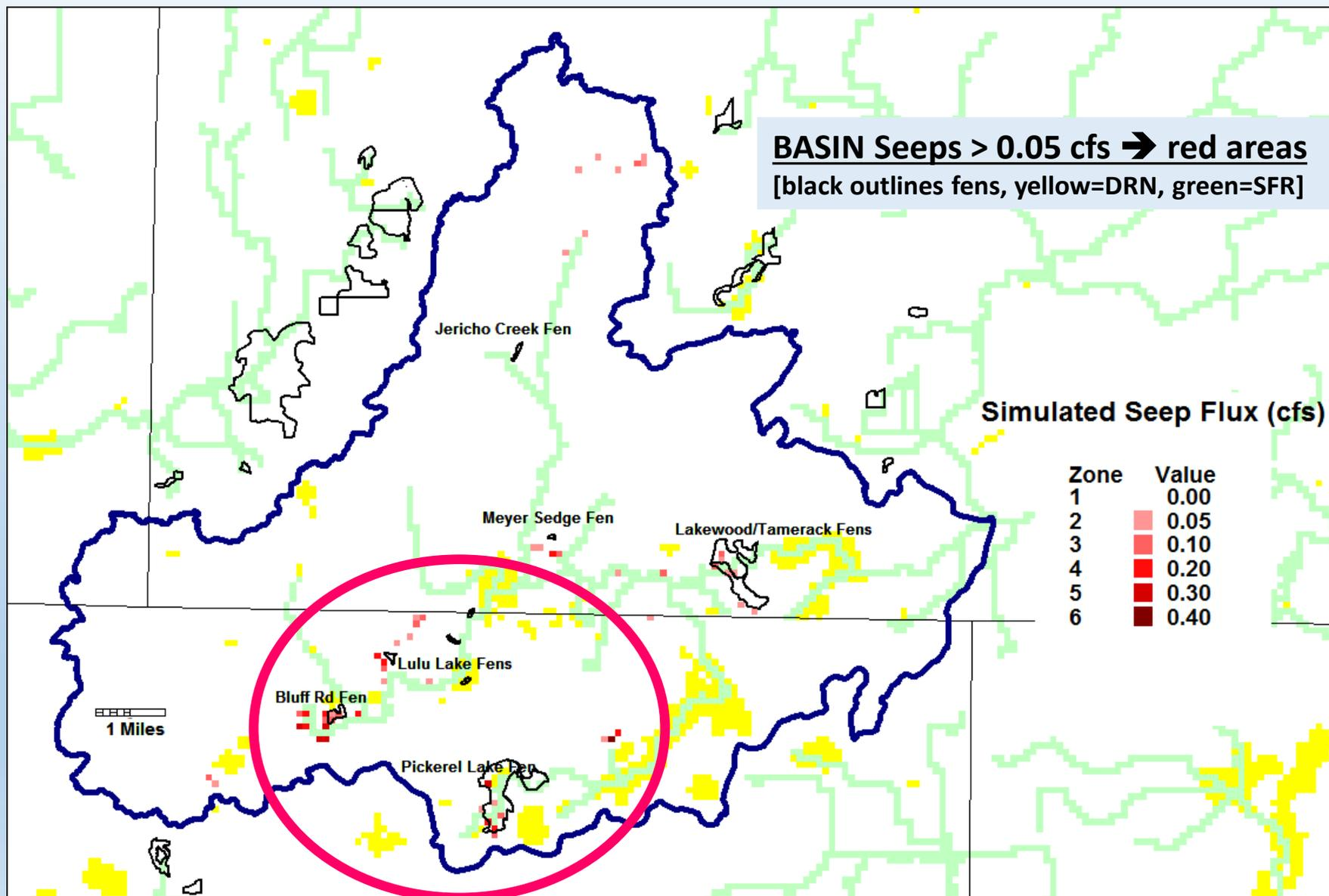
For our application: **Mean** land surface from 30m DEM for **500' x 500' cell worked best** (influences # of fen cells and rate of seepage)
